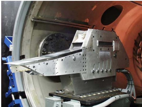
Note the windows in the side walls which permit visualization of the flow within the combustor
