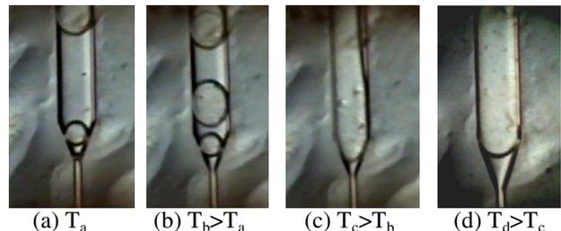
**Figure 3** - Evolution of the internal flow boiling patterns. Bubbles form at the expansion, grow to fill the downstream channel cross-section, then convect downstream (a). At higher wall temperatures, the frequency of bubble formation increases (b), reducing the spacing between them, until stable annular flow is achieved (c). Annular flow rapidly leads to completely evaporated stream downstream of the expansion as the temperature is increased further (d).
