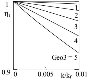
Fig. 3: Fin efficiency  $\eta_f(k/k_f, \text{Geo3})$  in relevant range (Equation 17)
