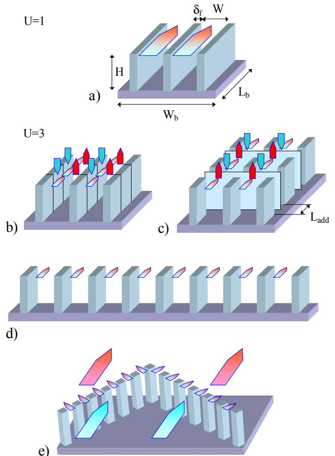
Fig. 1: Heat Sink configurations: a) regular finned base, b) fins divided in fin units with fresh coolant introduced into each unit, c) a longer base accounts for the space required for coolant inlet/outlet of each unit, d) side-by-side arrangement of fin units alleviates additional spacing for inlet/outlet, e) zigzag arrangements of the fin units can reduce overall pressure loss compared to c)
