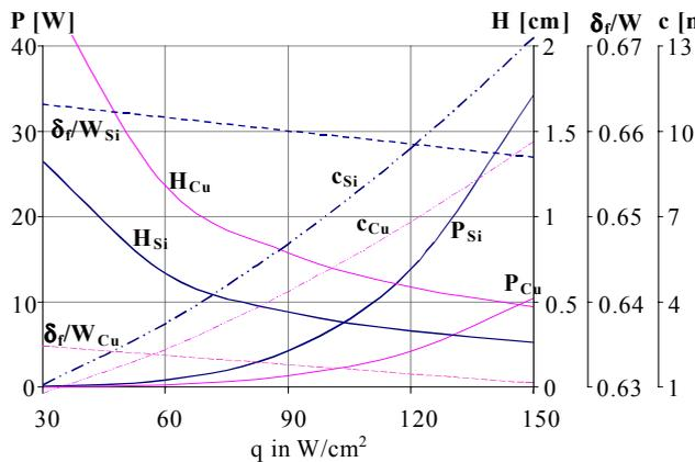
Fig. 11a: Optimized zigzag heat sinks: air cooled, approach temperature 32°C, base temperature 84.5°C, base area 1cm<sup>2</sup>, η=0.3
