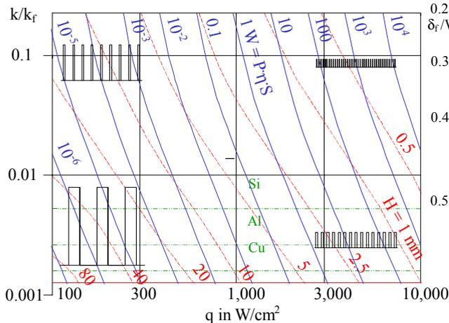
Fig. 8: Design chart for optimized heat sinks:
