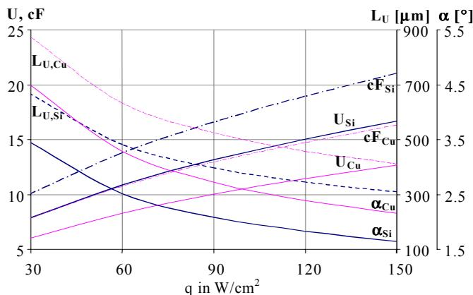
Fig. 11b: Optimized zigzag heat sinks: air cooled, approach temperature 32°C, base temperature 84.5°C, base area 1cm<sup>2</sup>, η=0.3
