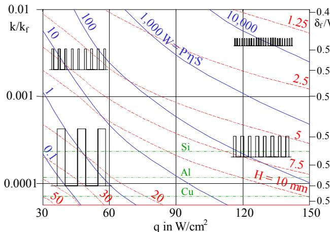
Fig. 7: Design chart for optimized heat sinks:
