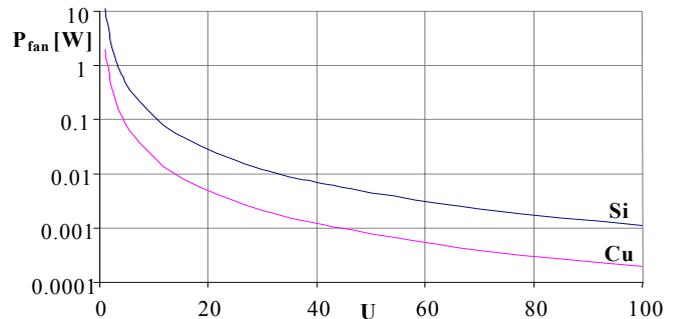
Fig. 6: Effect of Unit number  $U$  on fan power  $P$ :
