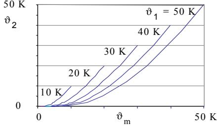
Fig. 2: Logarithmic mean temperature (Equation 7)
