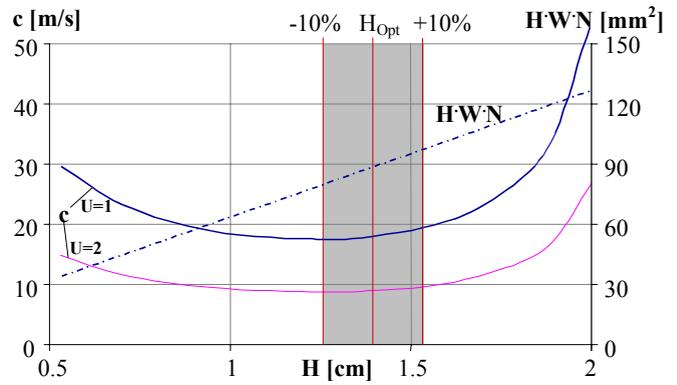
Fig. 5: Effect of fin height  $H$  on through flow velocity  $c$ :
