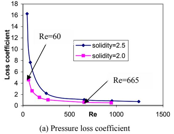
(a) Pressure loss coefficient
