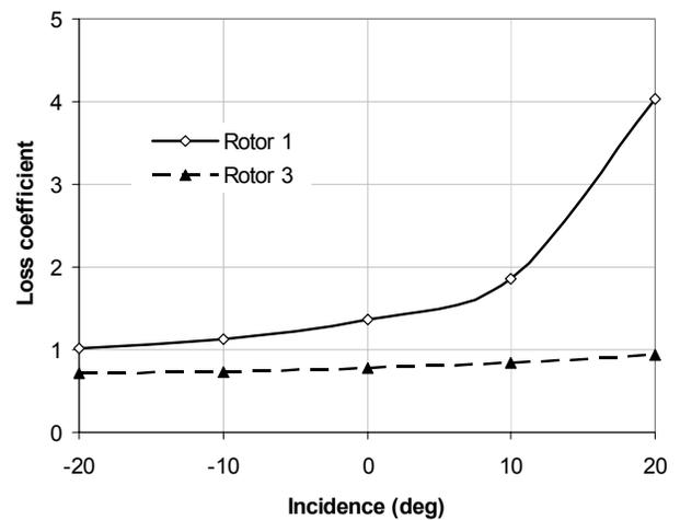
(a) Loss coefficient versus incidence
