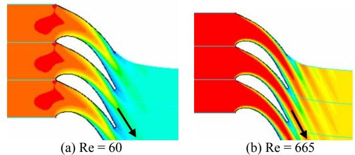
**Figure 6 - Total pressure contours for NACA A3K7 turbine stage with solidity of 2 (Rotor 3), showing that low Reynolds numbers (a) lead to thick boundary layers and slightly shallower exit flow angles.**
