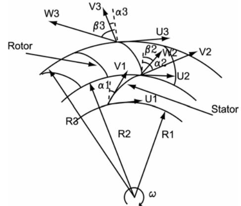
**Figure 2 – Velocity triangles in one turbine stage**
