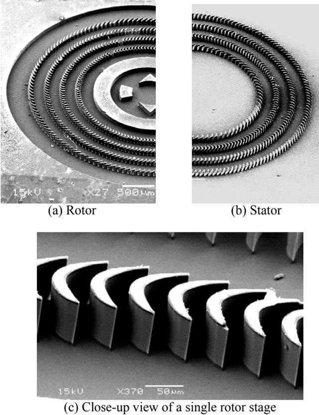
**Figure 1 - SEM image of a typical radial, multi-stage microturbine formed by DRIE, showing the rotors (a) and stators (b) on separate chips, as well as a close-up view of one blade row (c). The turbine is assembled by laying the stator chip over the rotor chip in order to interdigitated the concentric blade rows.**
