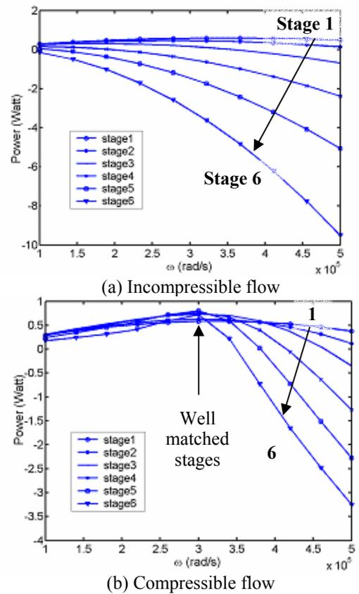
**Figure 3 - Power production per stage for a baseline microturbine (negative power indicated that the stage is adding work to the flow instead of extracting work) – baseline flow rate of 24 mg/s; 2mm diameter rotor.**
