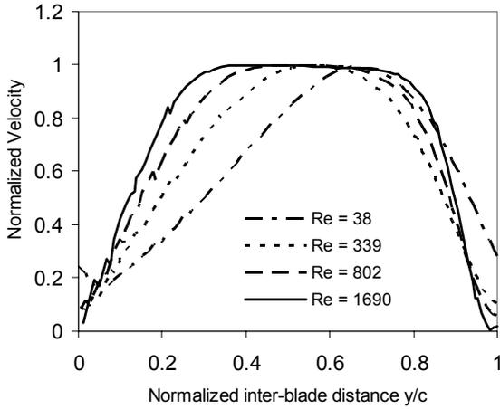
**Figure 7 - Profile of normalized velocity magnitude ( $V/V_{max}$ ) across the flow passage (Rotor 3), taken at 5% chord downstream of the blade row.**
