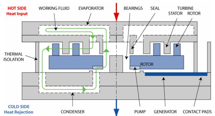
**Figure 2** - Cross-section schematic of micro steam-turbine power plant-on-a-chip. Constructed from 5 silicon wafers that are deep reactive ion etched and bonded to integrate the components on a single chip.
