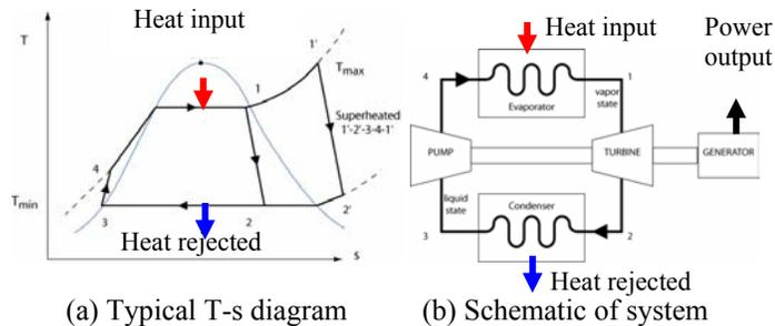
**Figure 1** - Standard superheated Rankine power cycle
