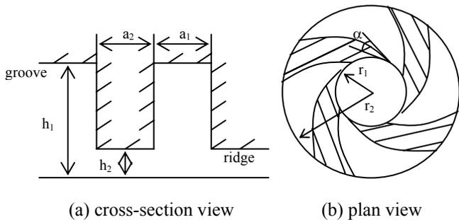
**Figure 6** - Spiral groove viscous pump configuration (less grooves are shown for clarity).
