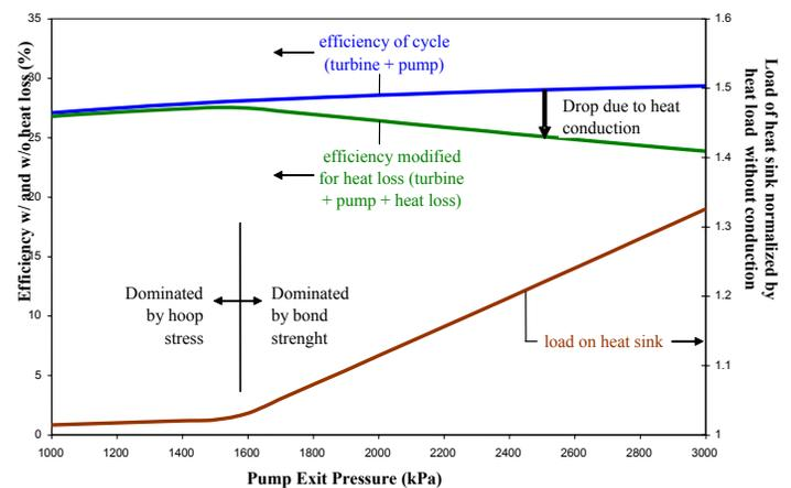
**Figure 11** - Impact of thermal conduction heat loss on cycle efficiency as a function of pump exit pressure. Although higher operating pressures improve the cycle efficiency, they require thicker walls to withstand pressure forces, and therefore increase the thermal leakage through the structure.
