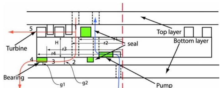
**Figure 8** - Cross-section schematic showing the liquid flow path (blue) and steam flow path (red) through the main and secondary flow components. A seal on the back side restricts the high pressure liquid to the inner radius, while the front side seal separates the high pressure steam and liquid. Axial balance is created by bleeding some of the turbine inlet steam under the disk, with the pressure controlled by the outer bearing.
