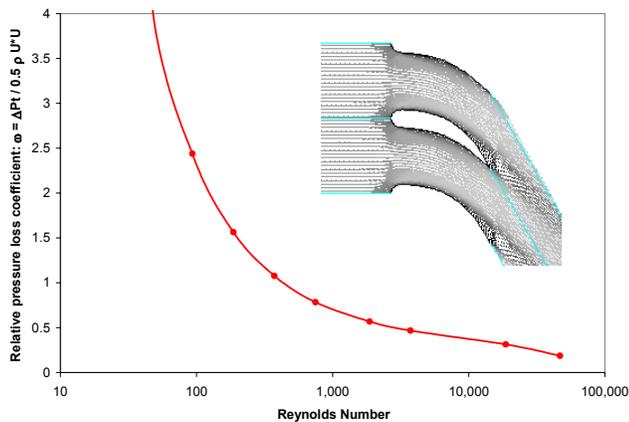
**Figure 12** - Relative pressure loss coefficient as a function of scale, represented by the Reynolds number.
