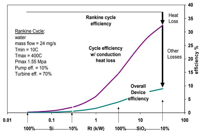
**Figure 10** - Impact of structural thermal resistance on efficiency, showing that a silicon junction between the hot and cold sides of the device leads to excessive drop in efficiency, but that small areas of silicon dioxide result in acceptable heat loss (percentages correspond to the ratio of wall area connecting the hot and cold sides to total chip area).
