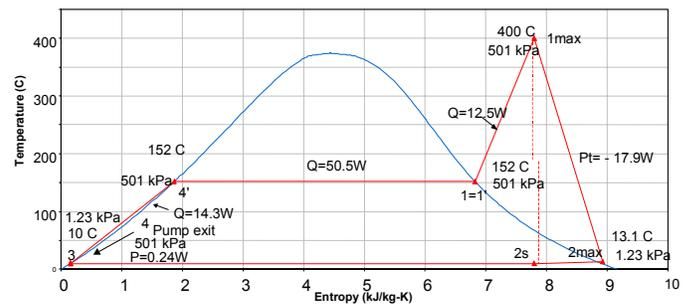
**Figure 4** - Temperature-entropy diagram of the Rankine cycle for typical design conditions (water, 24 mg/s,  $T_{min}=10^{\circ}\text{C}$ ,  $T_{max}=400^{\circ}\text{C}$ ,  $P_{max}=0.5\text{ MPa}$ ).
