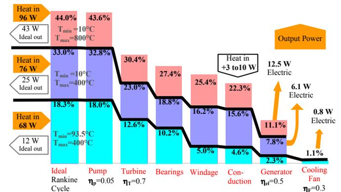
**Figure 9** - Predicted performance of the Micro Steam Turbine Power Plant-on-a-chip for three configurations. Bars illustrate the reduction in power as the various sources of loss in the system are incrementally considered, from left to right (water 24mg/s,  $P_{max}=0.6$  MPa).
