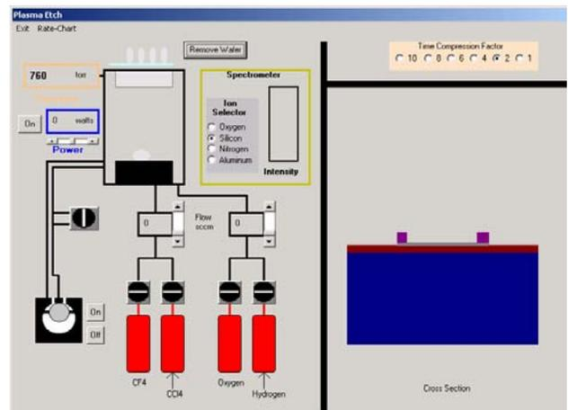
**Figure 2** Virtual plasma etch system.
