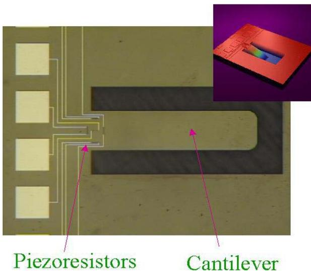
**Figure 3** Microscope and WYKO (inset) images of flow sensor. Resistors are  $10\ \mu\text{m}$  wide by  $200\ \mu\text{m}$  long.
