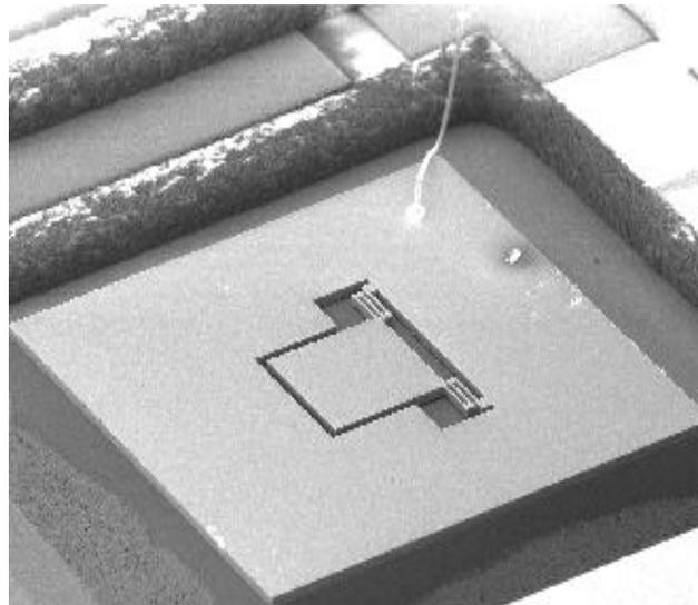
**Figure 4** SEM image of micro-actuator. The mirror plate is  $0.7\ \text{mm}$  on each side.
