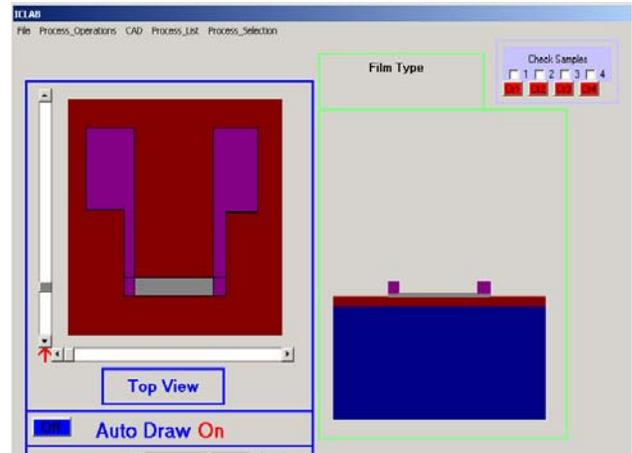
**Figure 1** Top and cross sectional views of polycrystalline silicon piezoresistor with aluminum leads on top of an oxidized silicon wafer.
