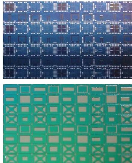
**Figure 5** Front and back of multi-device wafer.
