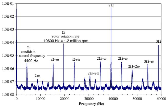
**Figure 6.** Power spectrum of the optical speed sensor signal showing the speed bump frequency ( $2\Omega$ ) and the rotor rotation rate ( $\Omega$ ), as well as other peaks corresponding to the natural frequency ( $\omega$ ) and its combinations with the rotation frequency.
