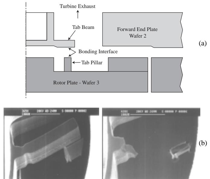
**Figure 5.** (a) Schematic of snap-off tab configuration. (b) SEM of bonded snap-off tab structures before and after fracture.
