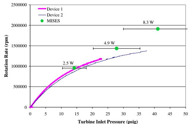
**Figure 8.** - Rotation rate as a function of the air pressure supplied to the turbine. There is a  $\pm 0.8$  psi uncertainty in the pressure.
