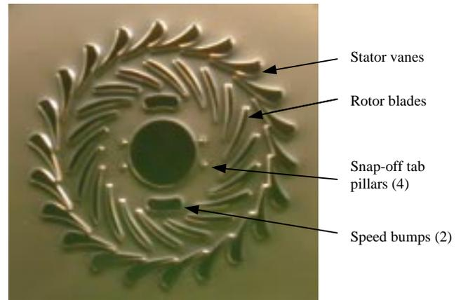
**Figure 3.** SEM of the 4.2 mm diameter microturbine showing the 150  $\mu\text{m}$  tall stator and rotor blades, two symmetric speed bumps, and four pillars for the snap-off tabs. In this picture, the journal bearing gap remains to be etched.
