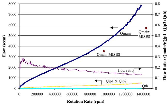
**Figure 9.** Turbine and bearing flow rates over the range of operating speeds for Device 2. Uncertainty in the main flow is  $\pm 200$  sccm, in the journal pressurization plenums (jp1 & jp2) is  $\pm 50$  sccm, and in the thrust balance plenum (tb) is  $\pm 0.5$  sccm.
