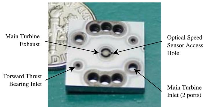
**Figure 1.** Microturbine-driven bearing rig die, consisting of a diced five-wafer bonded stack, which encloses a 4.2 mm rotor.
