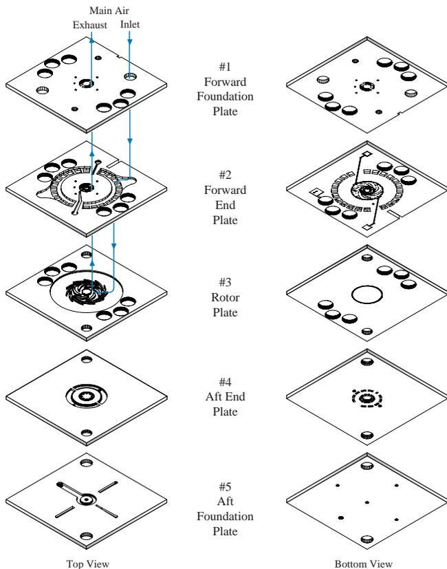
**Figure 4.** Top and bottom view of the five-stack device. The die is 15 mm per side and 2.3 mm thick.
